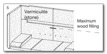
The fuel load, must be maintained below the top series of air holes and within the outer vent in each side. Fig. 5
