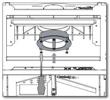
The flue collar is bolted to the stove from inside the fire chamber with, 4 x M6x10 0008-1117.
