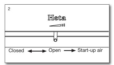
The Scan-Line Solid C stoves are designed and tested to burn extremely cleanly with very little smoke discharge and are exempt for use in smoke control areas throughout the UK when burning dry wood logs. To comply, a permanent stop is fitted to ensure that the air control slider cannot be closed beyond (percentage of air as per test) of its fully open position. A permanent
