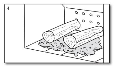
The wood will then ignite within a very short time (Typically 1 to 3 minutes). Once the fuel is Ignited. Close the door and regulate the air back to operating air. When the fire is well established, you can now regulate the operating air to the desired combustion level.
